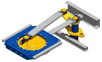
• Fifth wheel units length and transfer levers height are designed to match the trailers gooseneck
