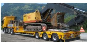
In contrast to mechanic and hydraulic steering systems, the EF-S system does not require a fifth wheel unit, but only a kingpin with integrated steering angle sensor. This creates a possible weight advantage, provided the required steering-energy is directly supplied by the truck, e.g. by hydraulic pump or alternator.
